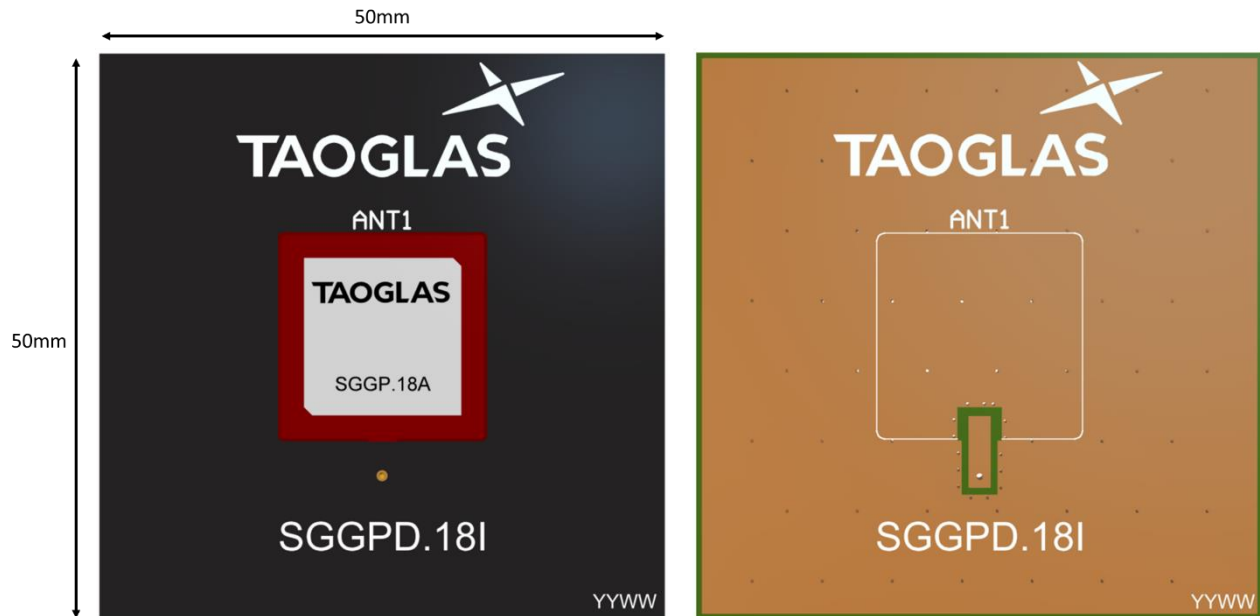
Top Side (SGGP.18.4.A.08 placement on 50x50mm PCB)
