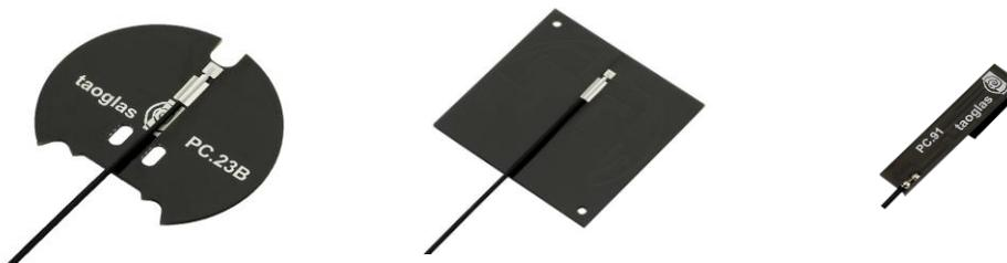
FR4 standard thickness is 0.8mm. Thicknesses of 1.6mm or other custom thicknesses of the laminate are available for custom projects.
